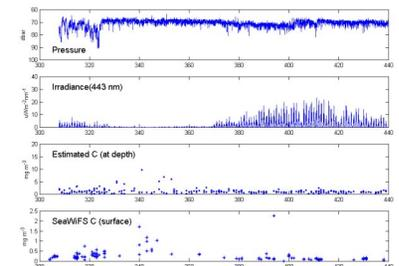
Figure 4: Data from an optical mooring deployed in the Southern Ocean in 1997 compared with SeaWiFS data. The data shown, from top to bottom, are the pressure variations experienced by the sensor, the measured downwelling irradiance at 443 nm, the estimated chlorophyll concentration at the sensor depth near solar noon using the derived method, and the surface chlorophyll concentration derived from SeaWiFS LAC and GAC data in the vicinity, respectively.
