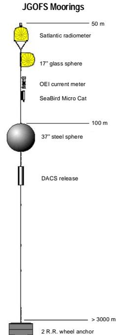
Figure 1: Schematic of optical moorings deployed in the Southern Ocean. Courtesy of David Reinert (Oregon State University).
